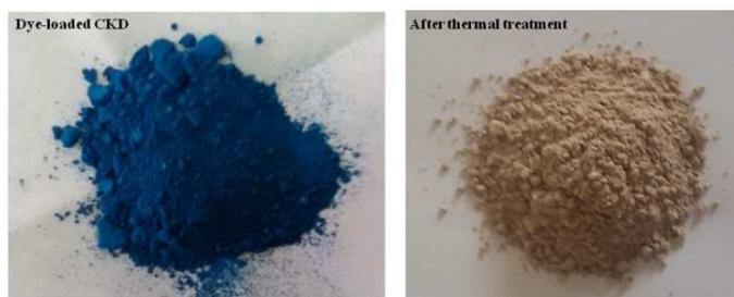
**Figure 11: Effect of Thermal Treatment on Dye-Loaded CKD**
